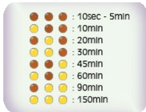
Figure 3 – Mapping table combination Led, with maximum continuous flow time (MCFT).
